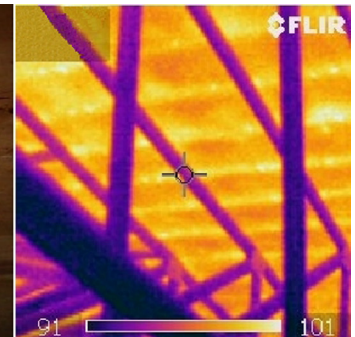
5/13/09 New roof tile over Therma Sheet. Span of IR image reduced to 91-101° F to match original 4/7/09 image. Attic temperature has been lowered 30°F with the addition of Therma Sheet.
